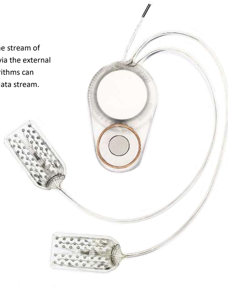
CorTec Brain Interchange currently features 32 channels, all of which can be used for recording and stimulation. No skin breach is involved due to its fully wireless functionality.
