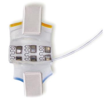
The innovation in CorTec's split cylinder cuffs is their flexible structure: The contacts are divided into two parts, allowing the cuff to be stretched to a certain extent without exposing the contact to tensile forces. The electrode can be removed without affecting its functionality.
