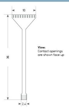
Polyimide technology allows the manufacturing of cuff electrodes as well. The following design can be used for recording and stimulation. It will be wrapped around the nerve with a diameter of 200 µm.
